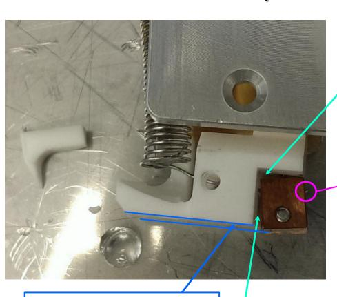
The base plane of the macor retainer is intended to be flush with the base plane of the macor retainer of the adjacent (upper) RH assembly.
