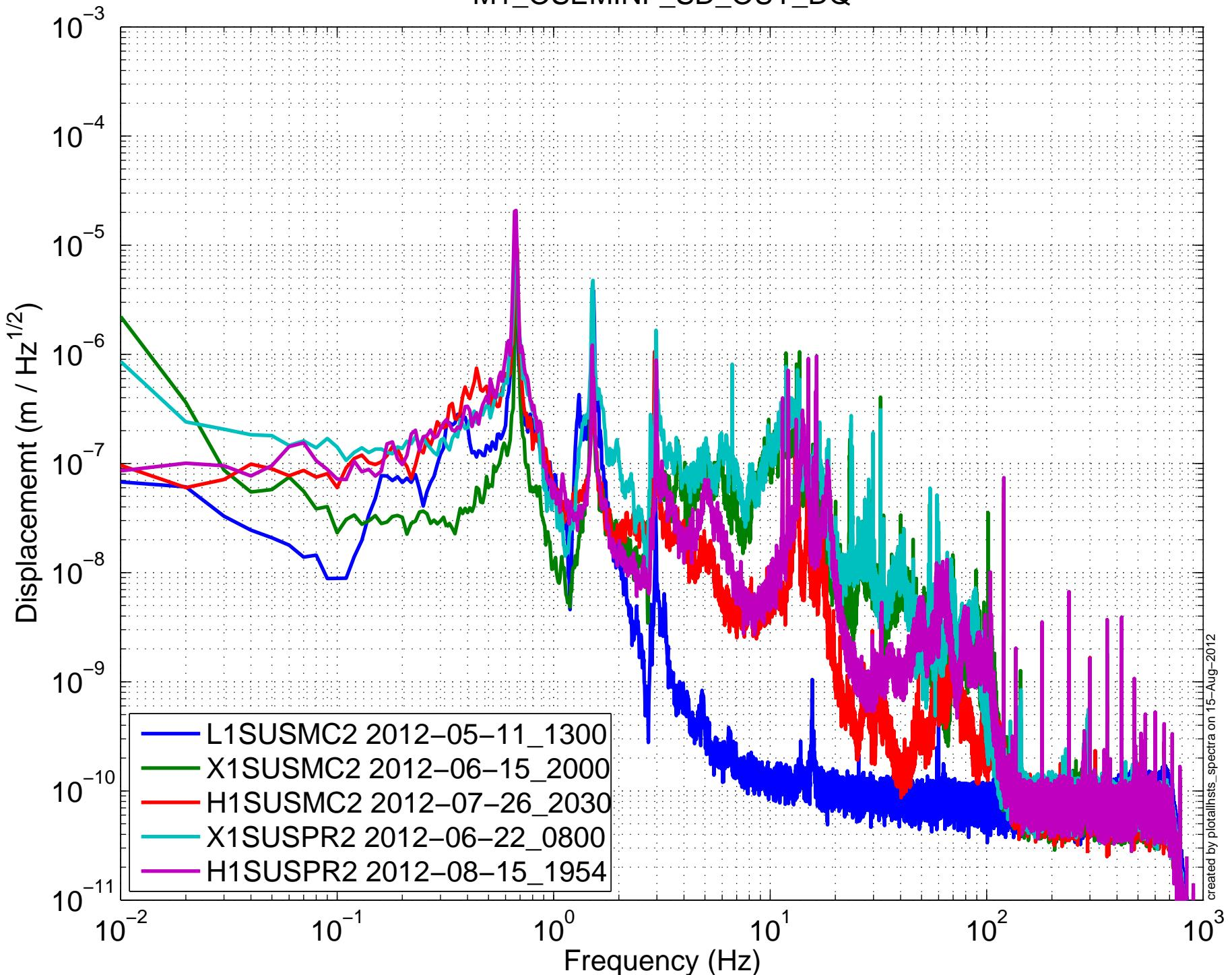
(HSTS) Amplitude Spectral Density – Damping OFF
