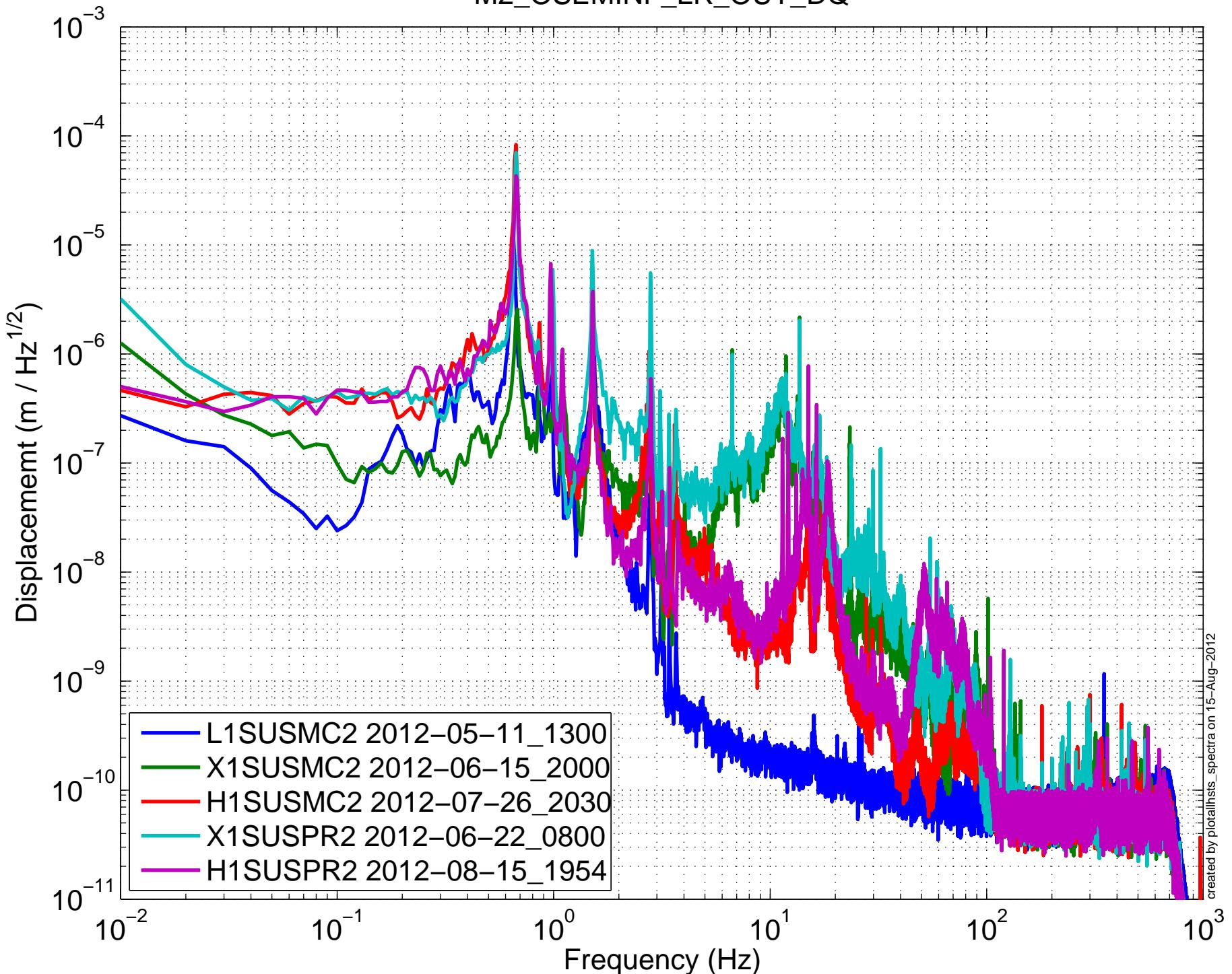
(HSTS) Amplitude Spectral Density – Damping OFF
