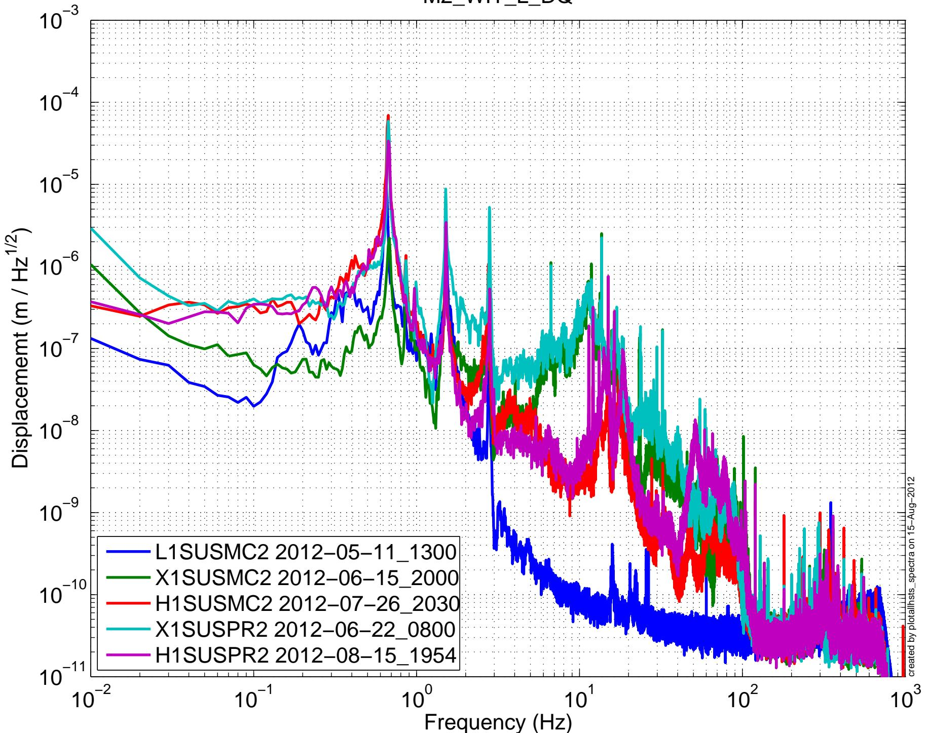
(HSTS) Amplitude Spectral Density – Damping OFF
