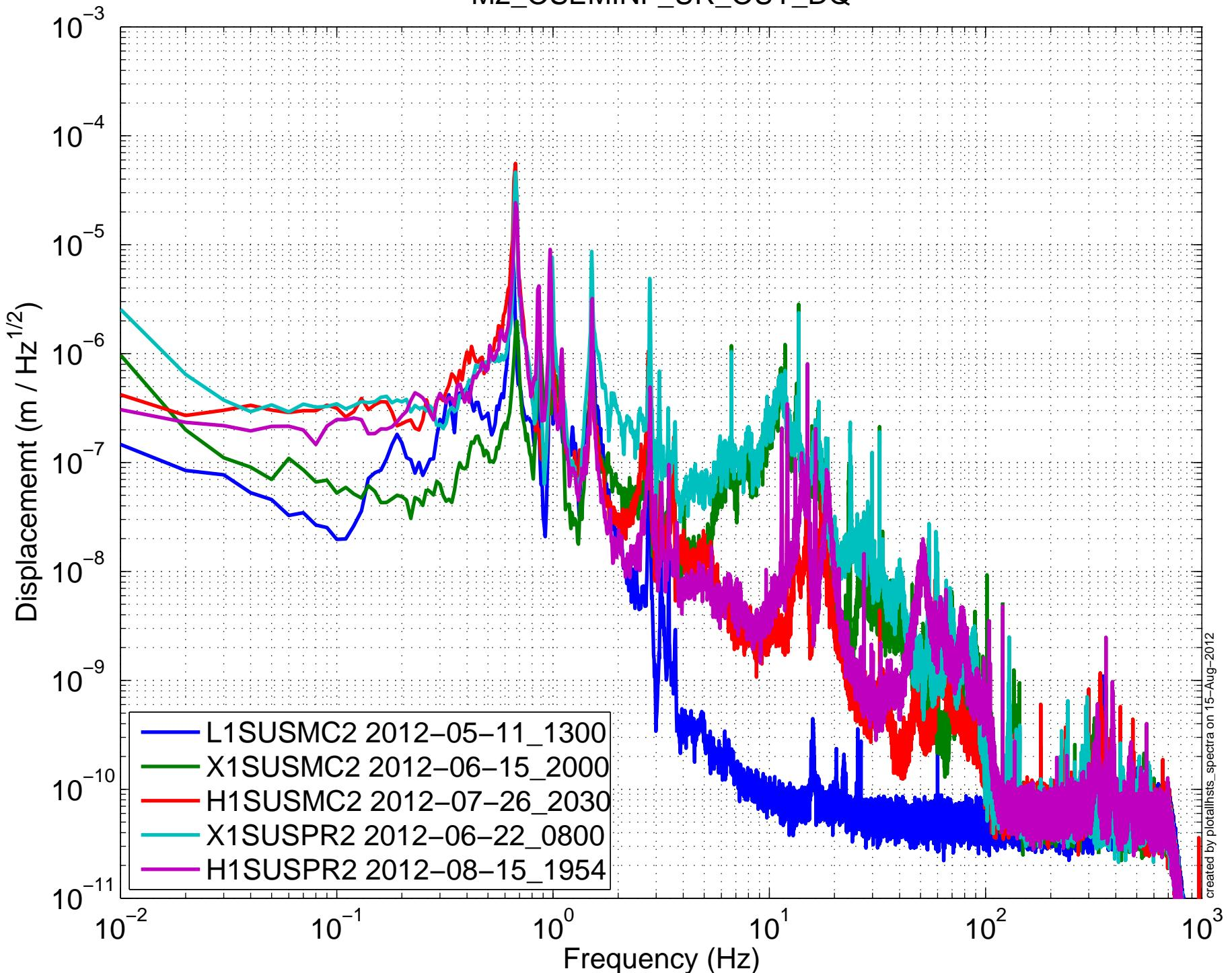
(HSTS) Amplitude Spectral Density – Damping OFF
