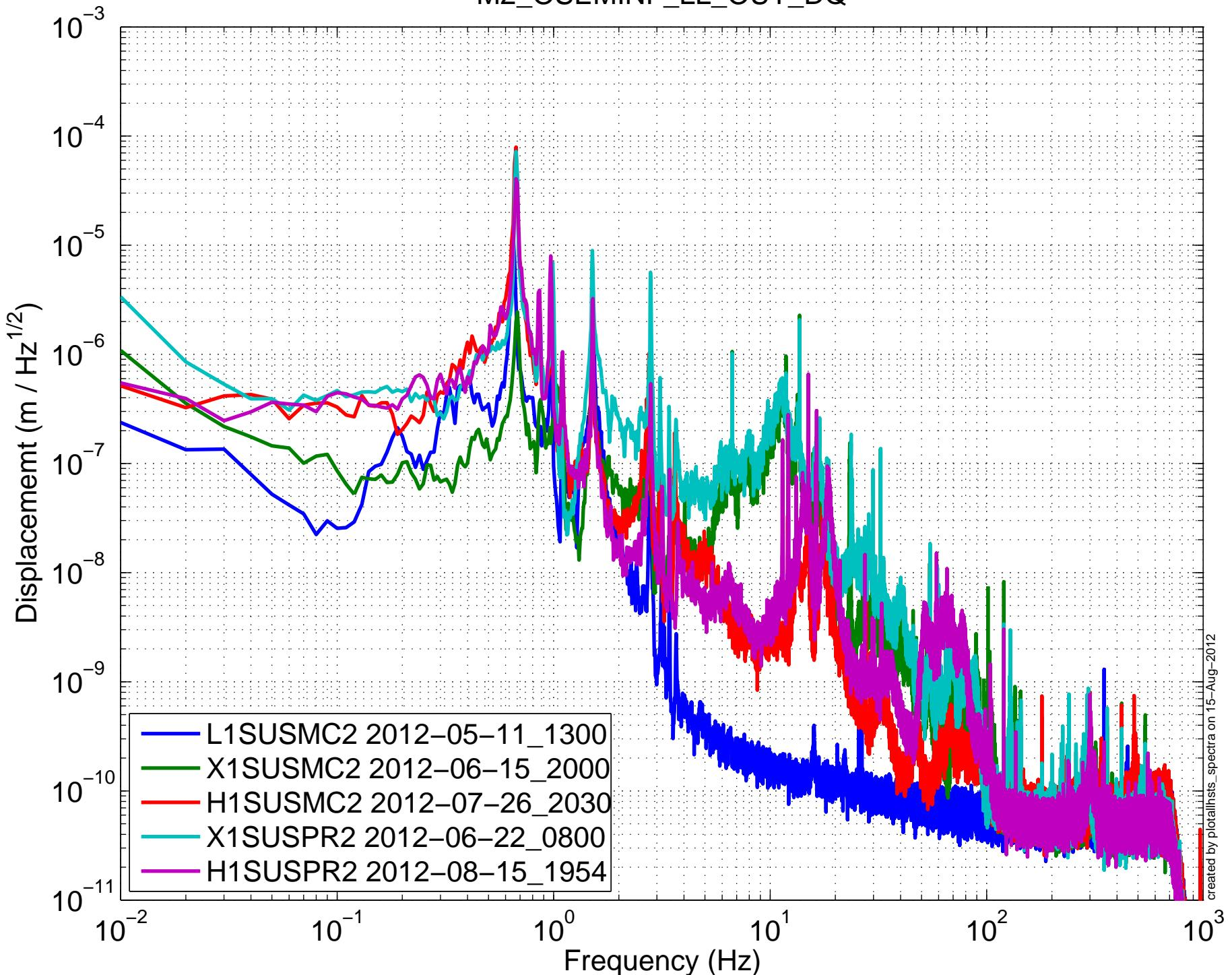
(HSTS) Amplitude Spectral Density – Damping OFF
