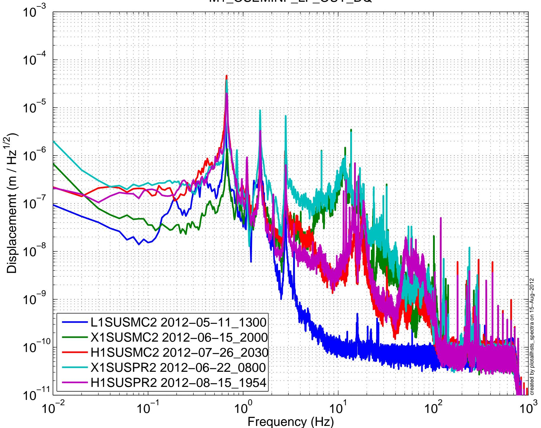
(HSTS) Amplitude Spectral Density – Damping OFF
