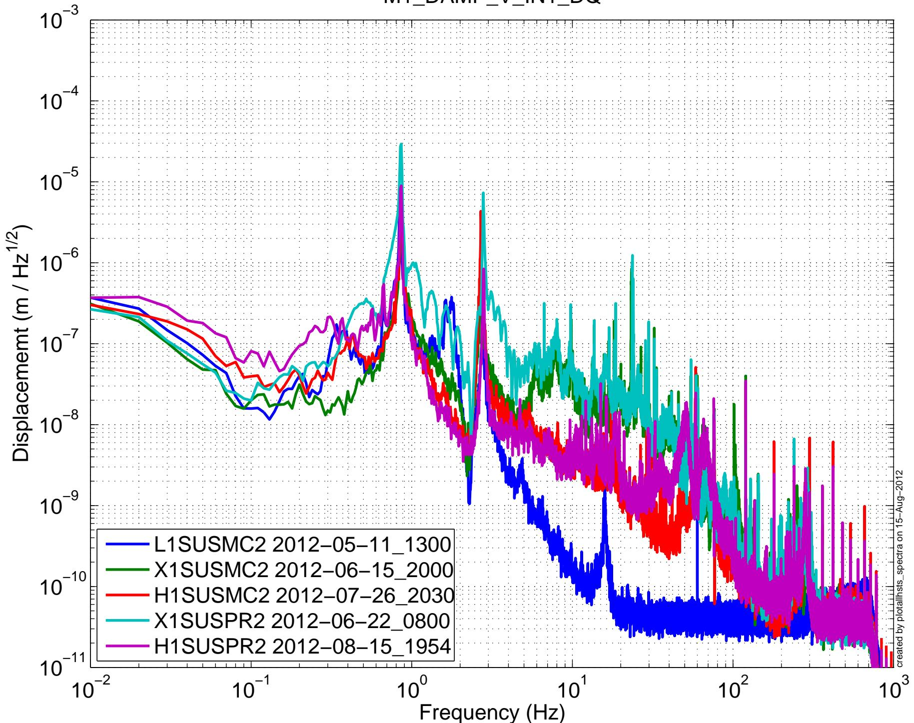
(HSTS) Amplitude Spectral Density – Damping OFF
