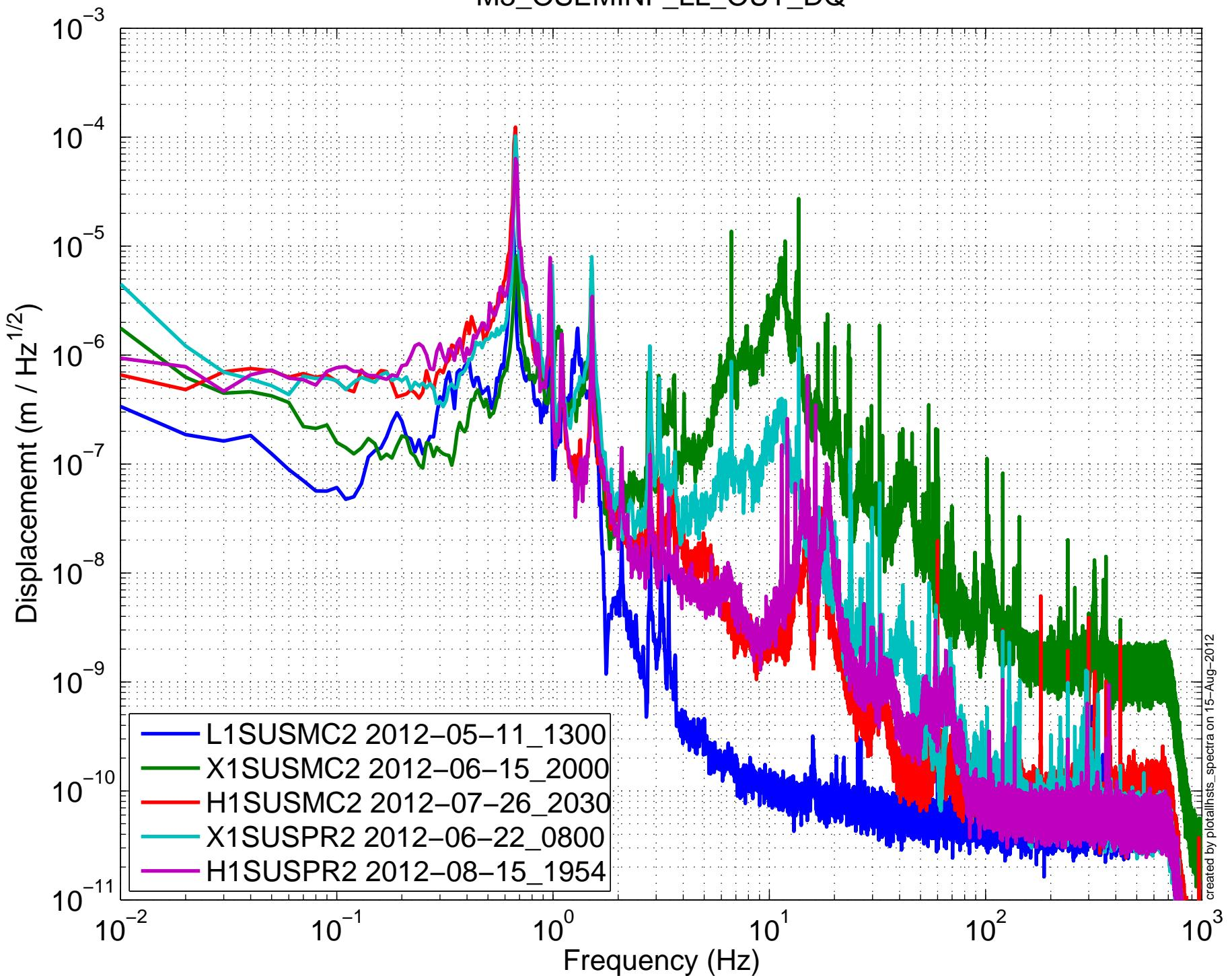
(HSTS) Amplitude Spectral Density – Damping OFF
