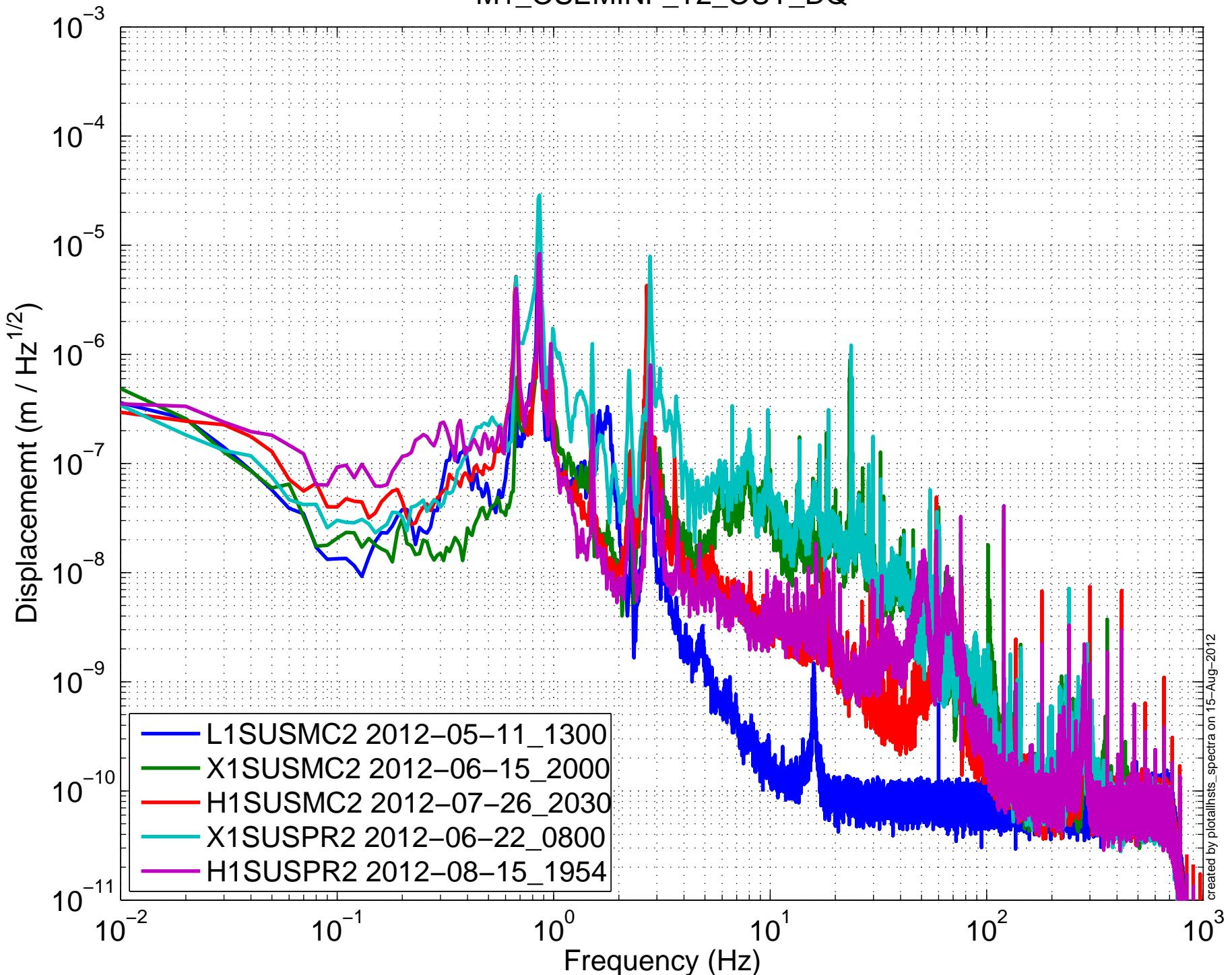
(HSTS) Amplitude Spectral Density – Damping OFF
