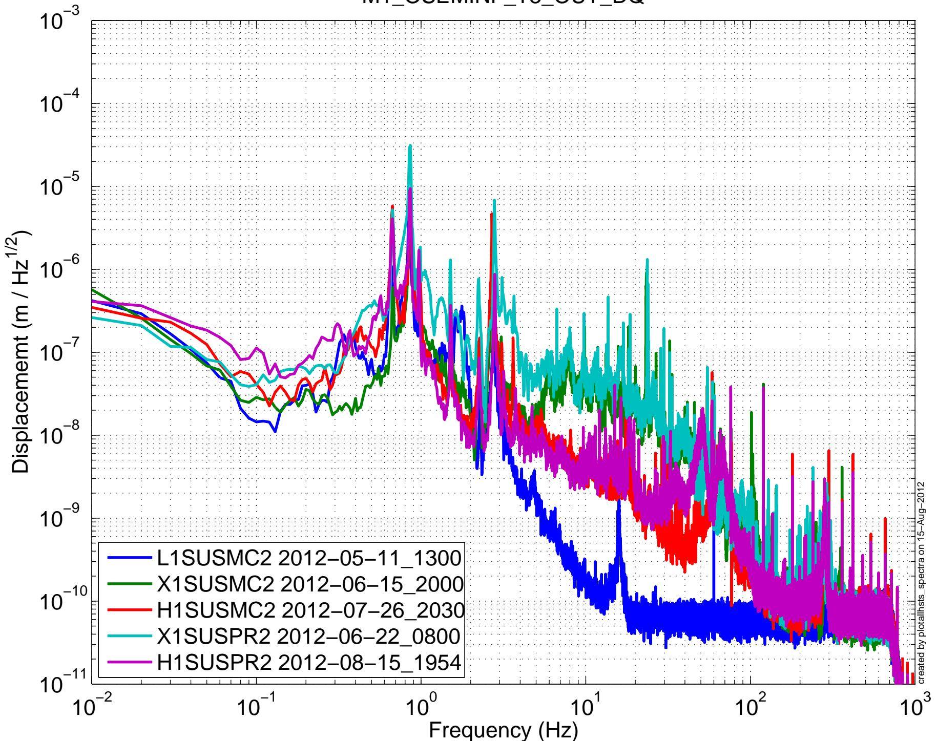
(HSTS) Amplitude Spectral Density – Damping OFF
