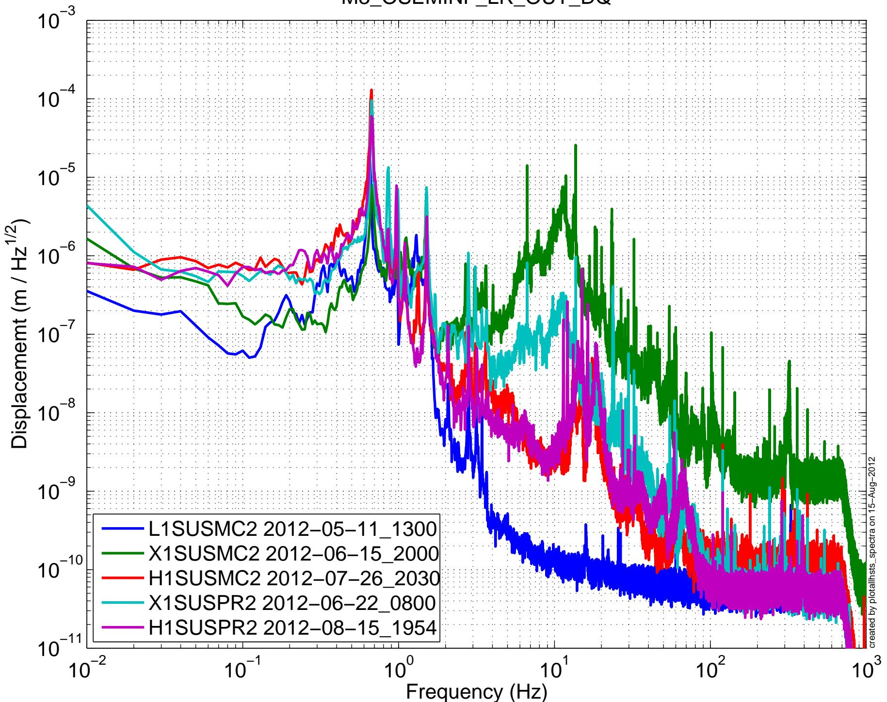
(HSTS) Amplitude Spectral Density – Damping OFF
