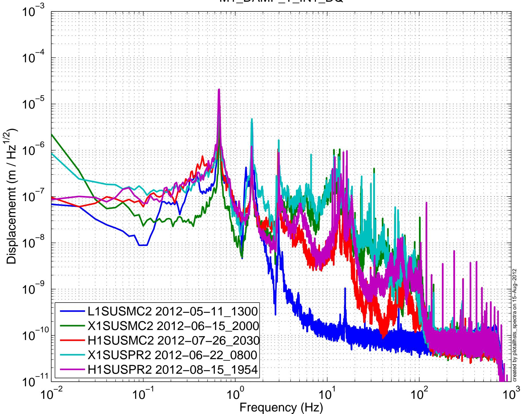
(HSTS) Amplitude Spectral Density – Damping OFF
