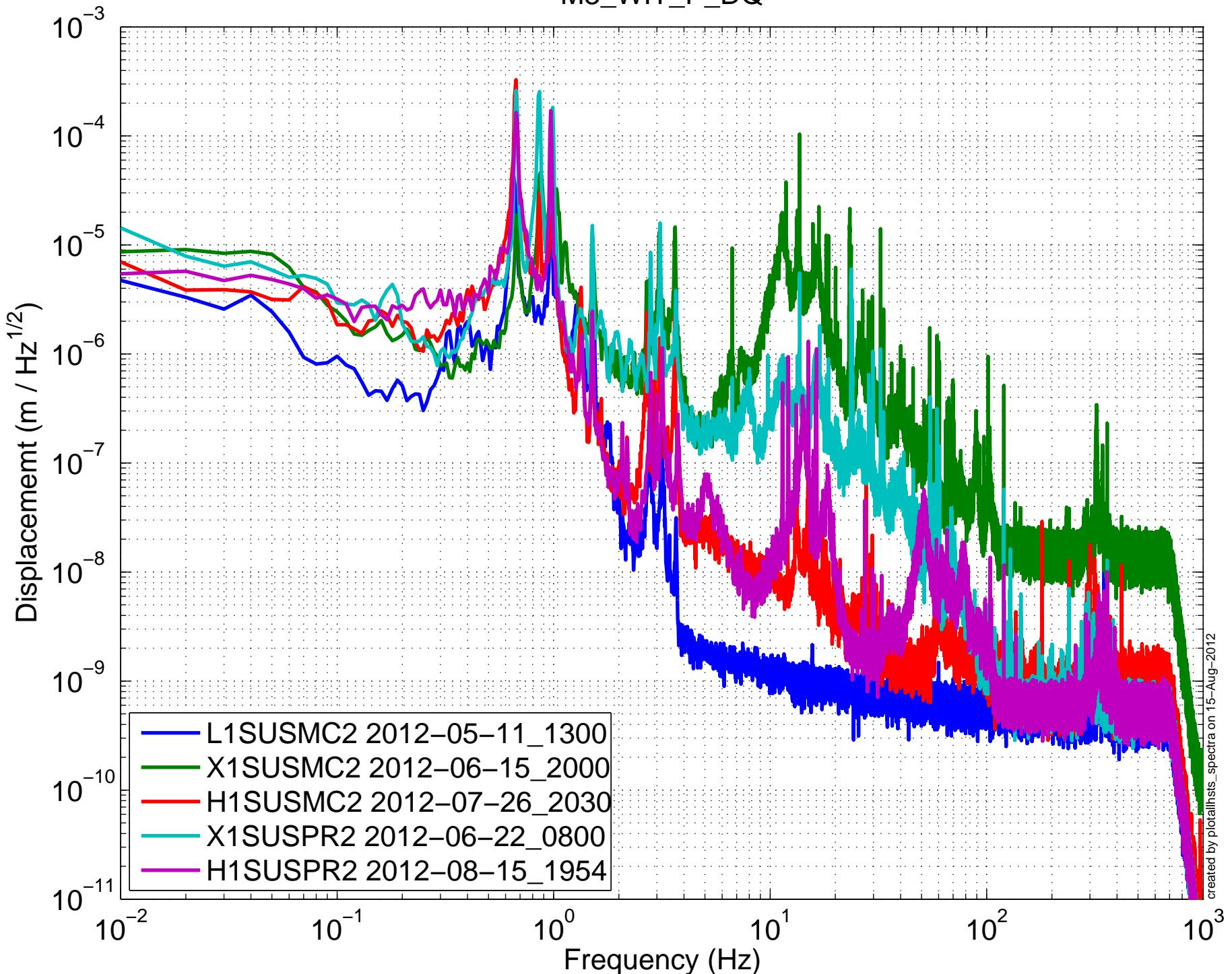
(HSTS) Amplitude Spectral Density – Damping OFF
