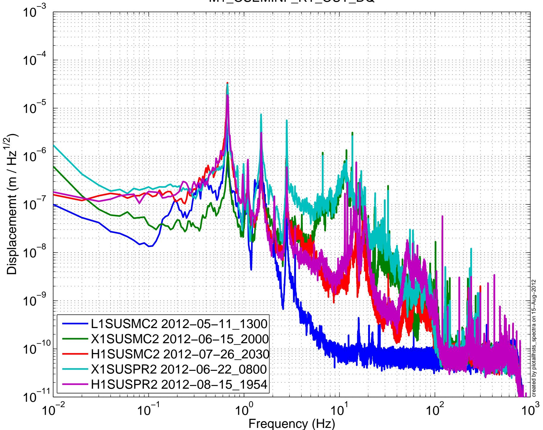
(HSTS) Amplitude Spectral Density – Damping OFF
