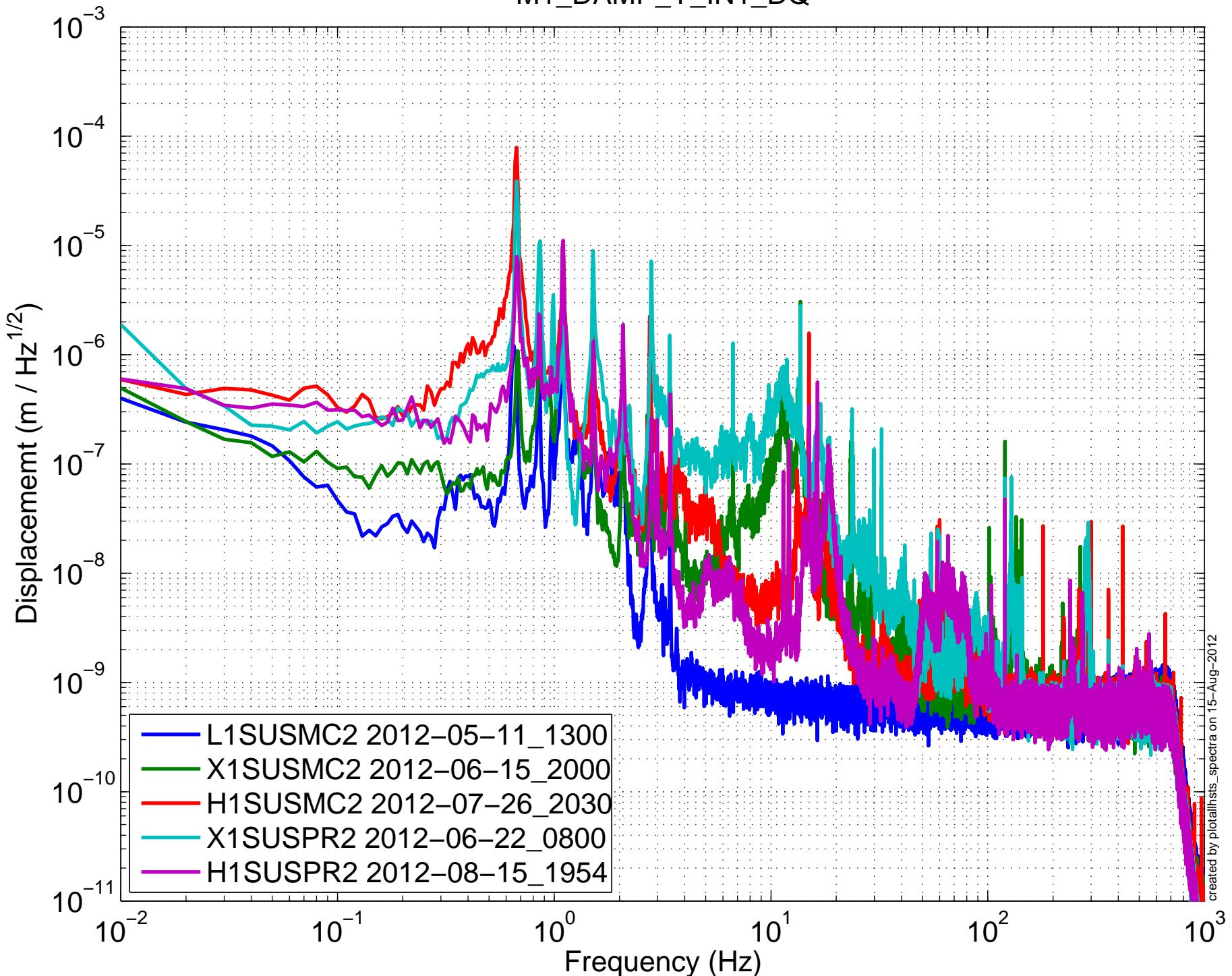
(HSTS) Amplitude Spectral Density – Damping OFF
