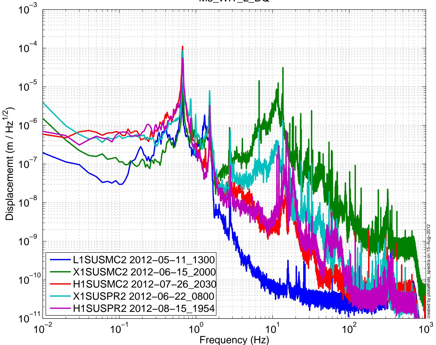
(HSTS) Amplitude Spectral Density – Damping OFF
