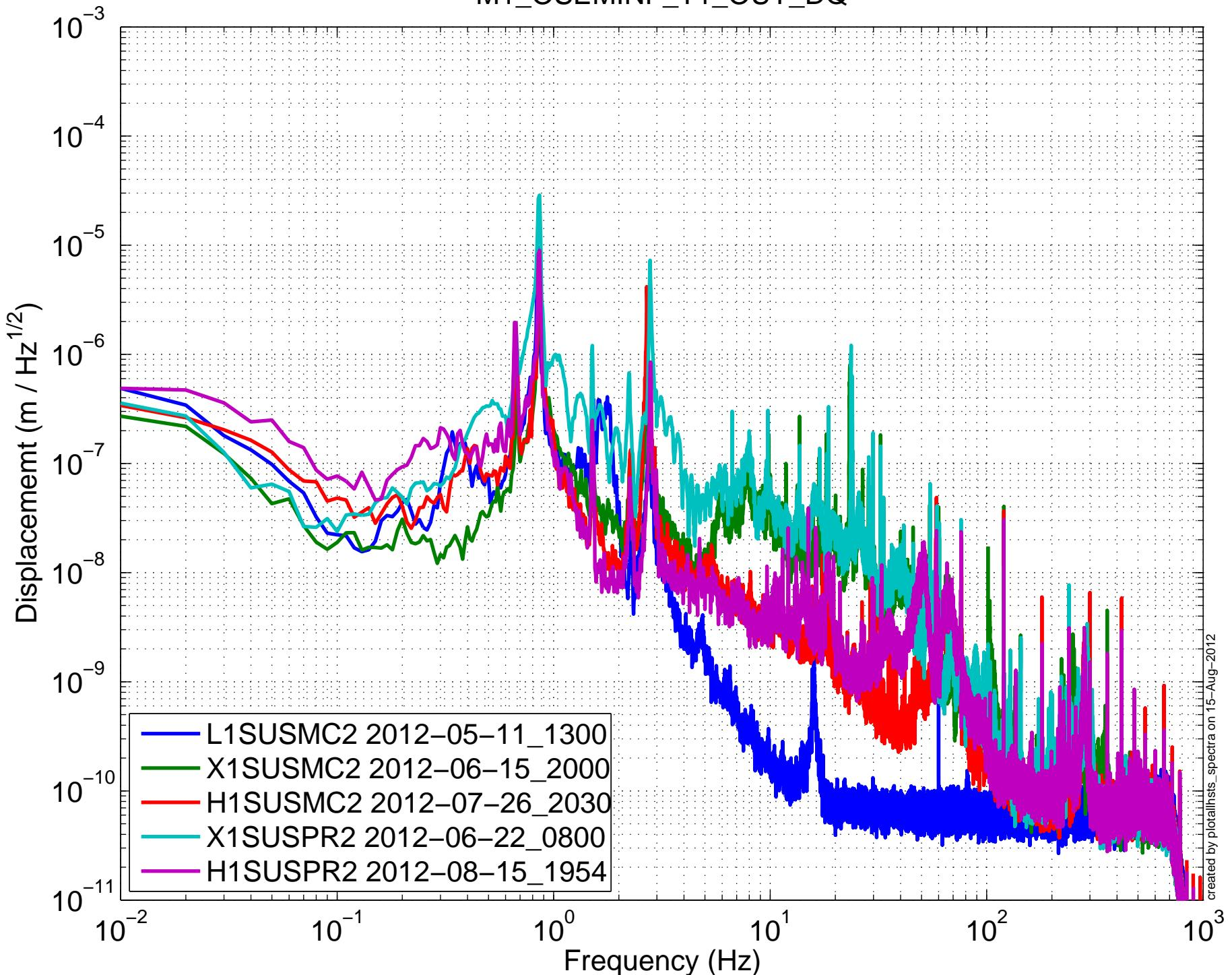
(HSTS) Amplitude Spectral Density – Damping OFF
