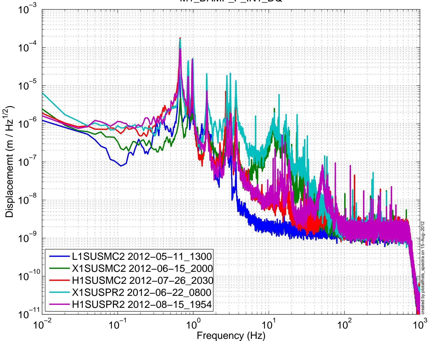
(HSTS) Amplitude Spectral Density – Damping OFF
