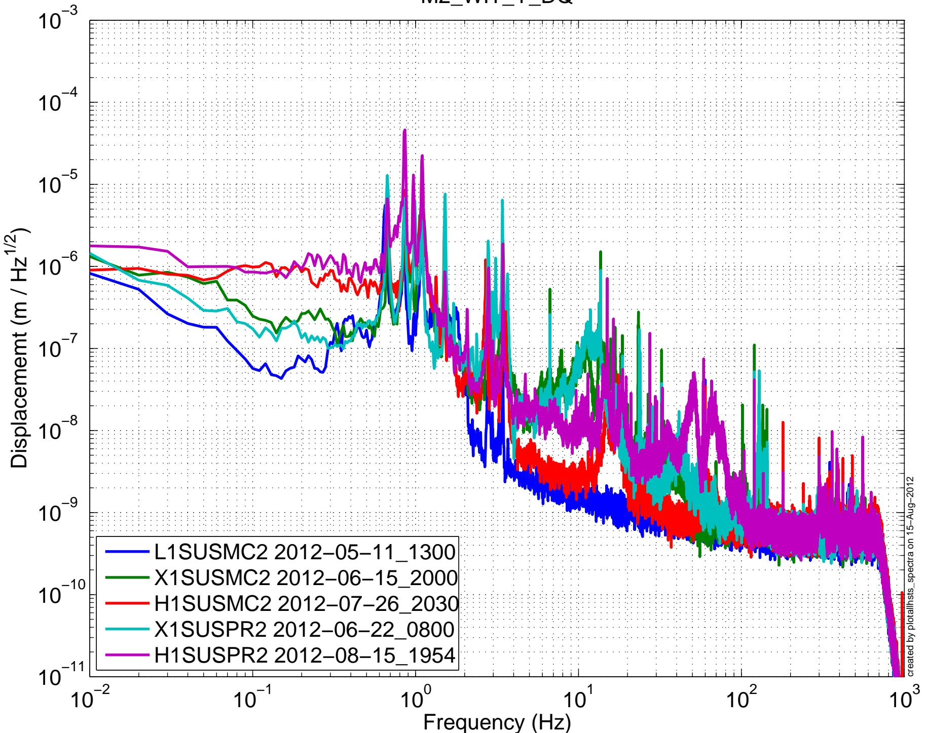
(HSTS) Amplitude Spectral Density – Damping OFF
