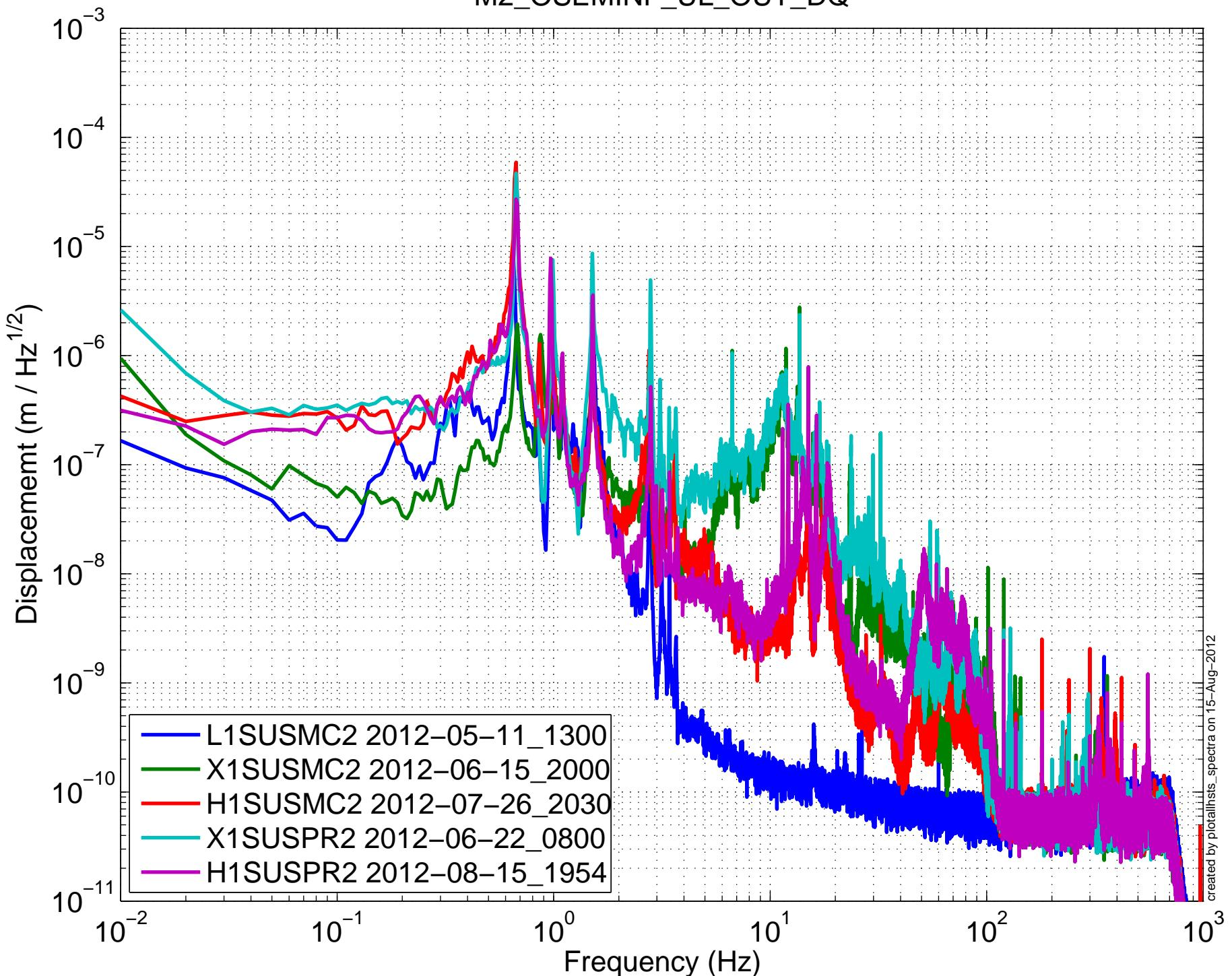
(HSTS) Amplitude Spectral Density – Damping OFF
