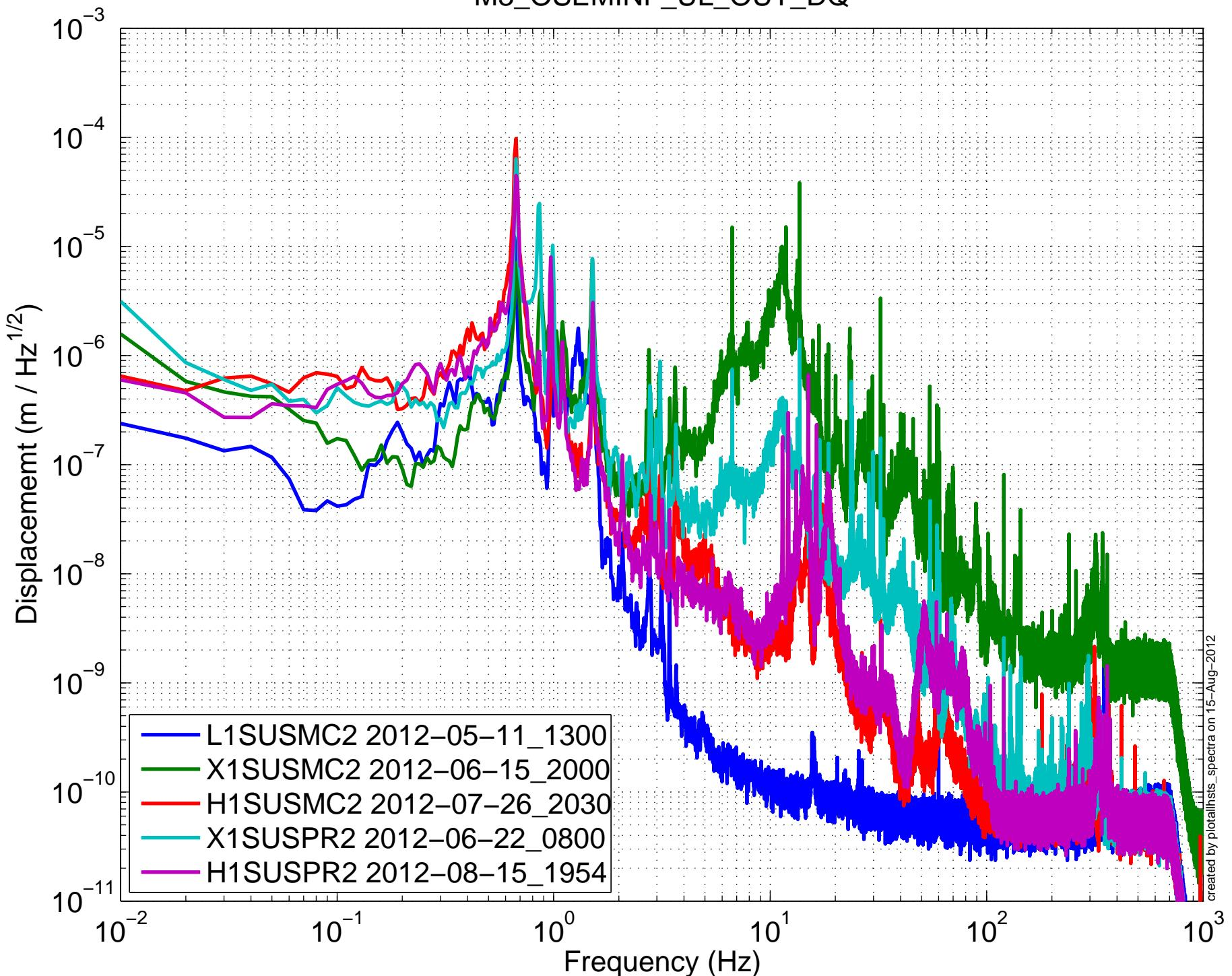
(HSTS) Amplitude Spectral Density – Damping OFF
