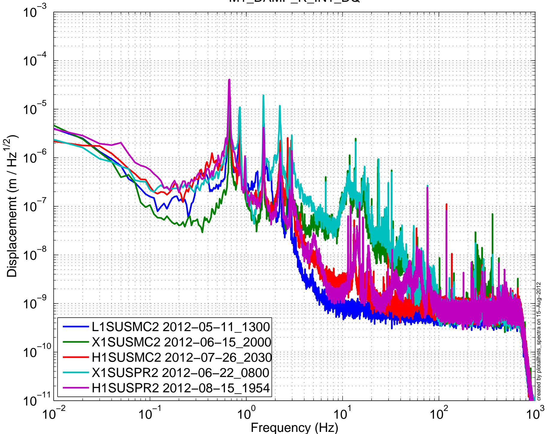
(HSTS) Amplitude Spectral Density – Damping OFF
