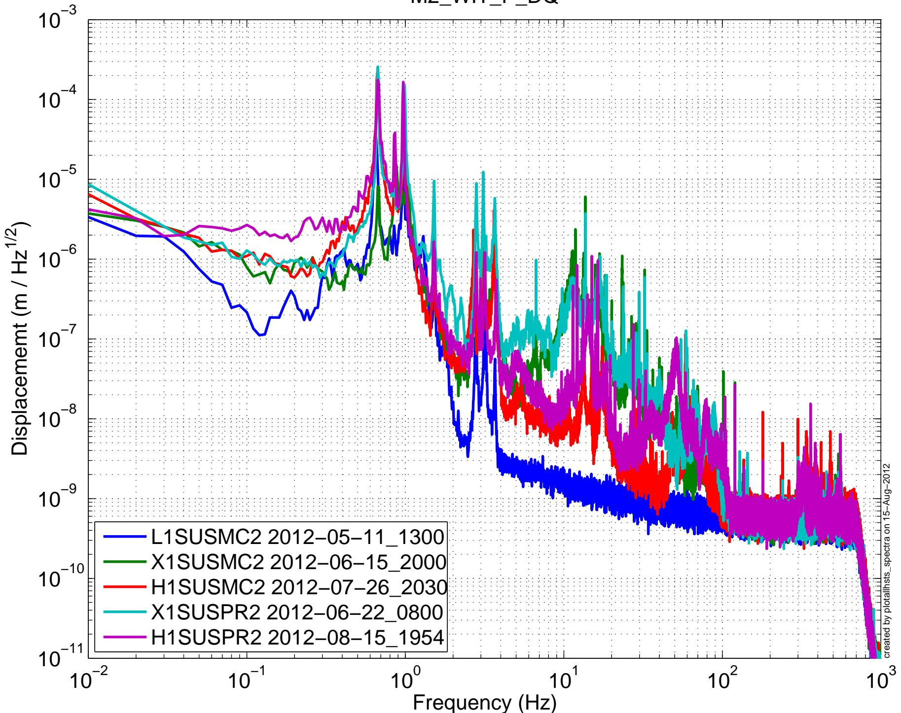
(HSTS) Amplitude Spectral Density – Damping OFF
