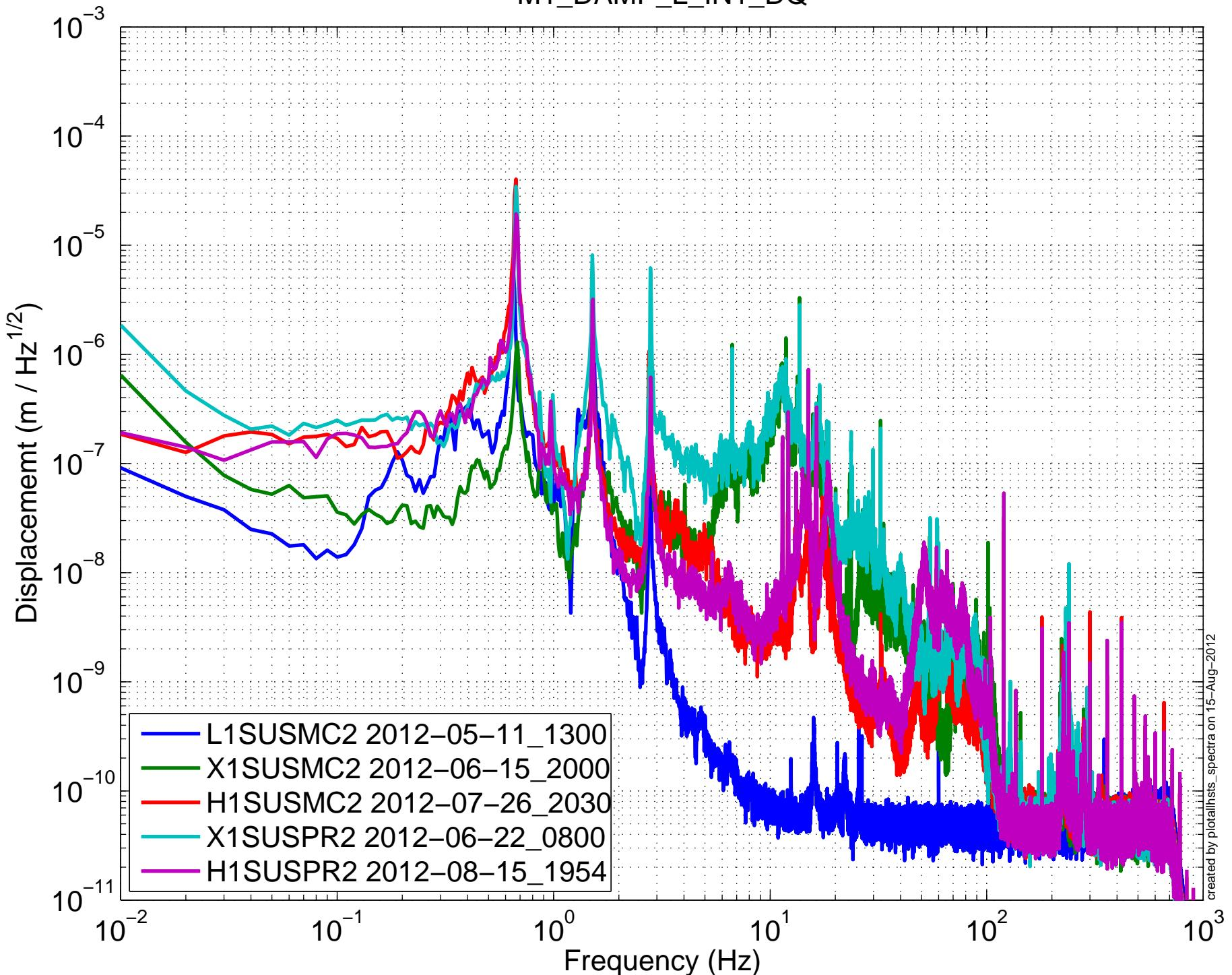
(HSTS) Amplitude Spectral Density – Damping OFF
