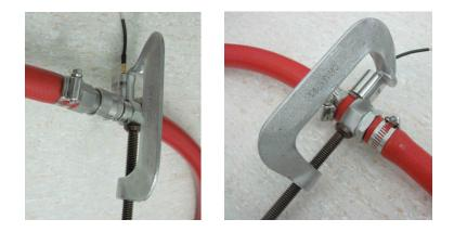
The quick connect on the left was ~100 times as noisy as the straight-through barrel connector on the right even though the flow (10 - 15 l/m) was probably greater for the lower resistance barrel connection. Data shown in the lower plot of Figure 1.
