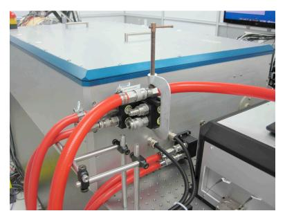
The quick connect clamped to the manifold for the top plot of Figure 1. Flow was 10 to 15 l/m.
