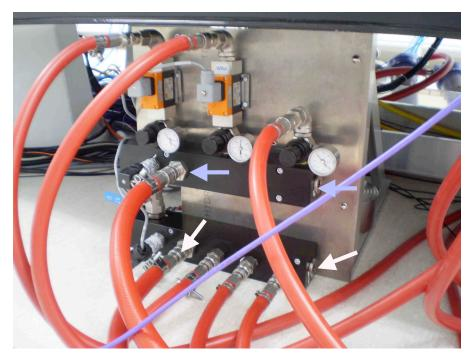
No further measureable improvements were made with these changes, but these changes may reduce laser jitter etc. Four hoses indicated by colored arrows were moved to burred connectors installed in the capped hole indicated by the same color arrow. The bottom picture shows the final configuration.
