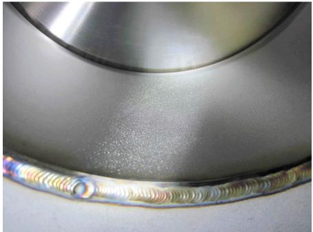
Top 2 photos are of nozzles in the 2K IMC tube. Bottom photo is of a nozzle in HAM3. There is much less particulate in the nozzle suggesting that vacuum cycling is not redistributing the particulate rapidly.
