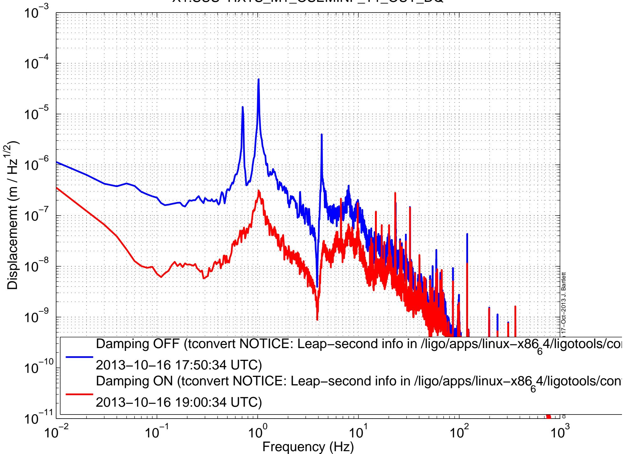
X1SUSOMC (OMCS) Amplitude Spectral Density
