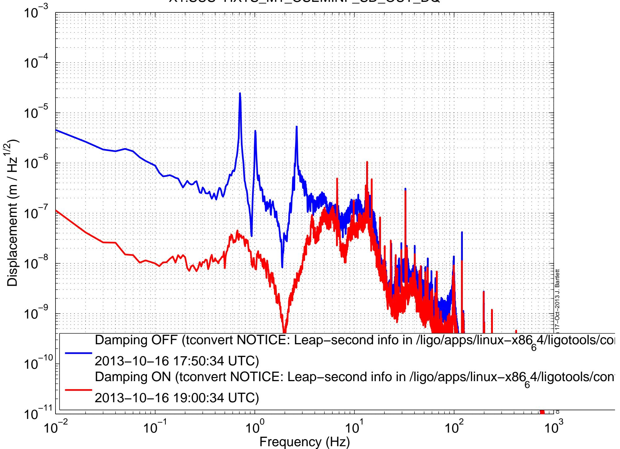
X1SUSOMC (OMCS) Amplitude Spectral Density
