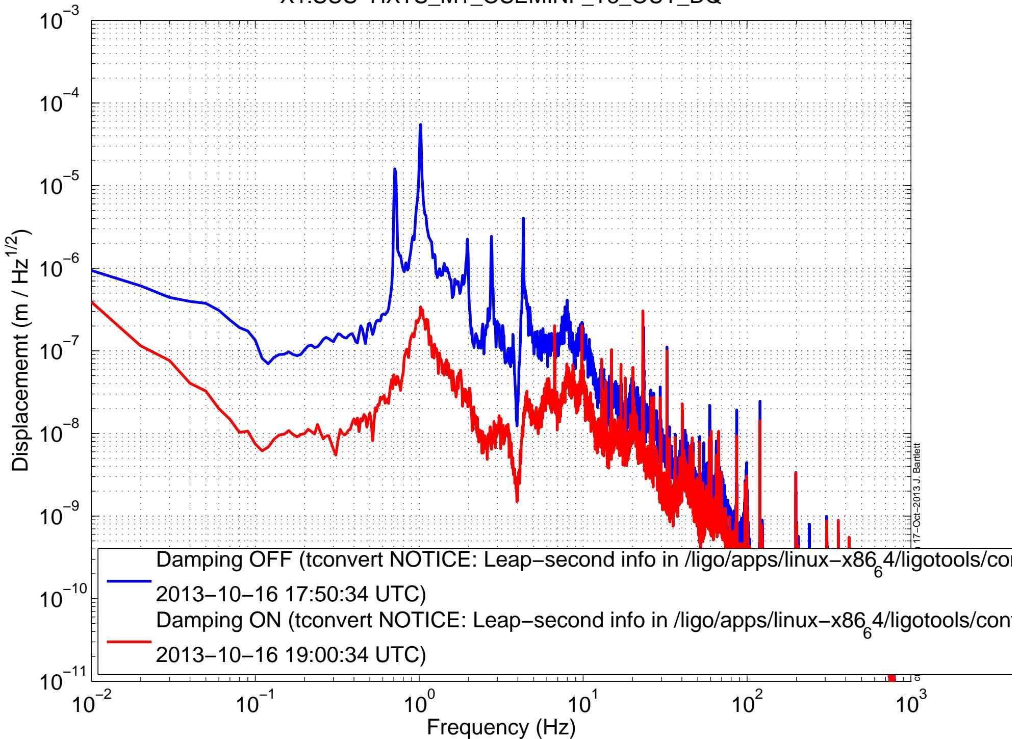
X1SUSOMC (OMCS) Amplitude Spectral Density
