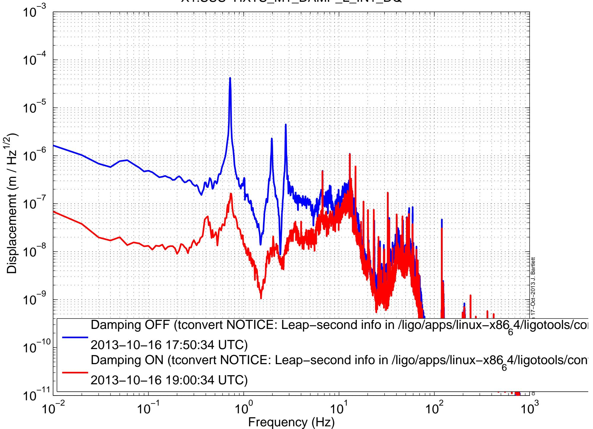
X1SUSOMC (OMCS) Amplitude Spectral Density
