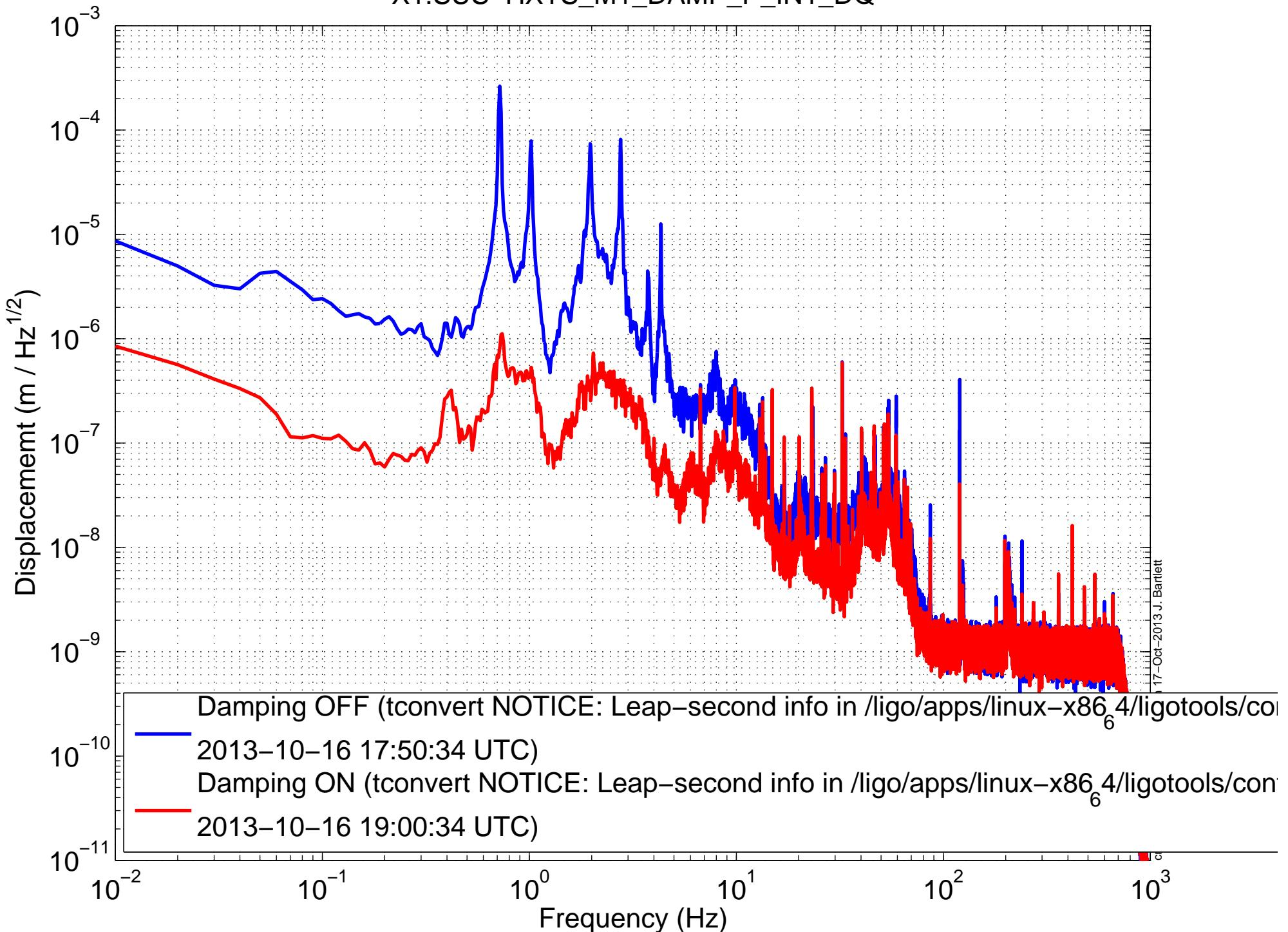
X1SUSOMC (OMCS) Amplitude Spectral Density
