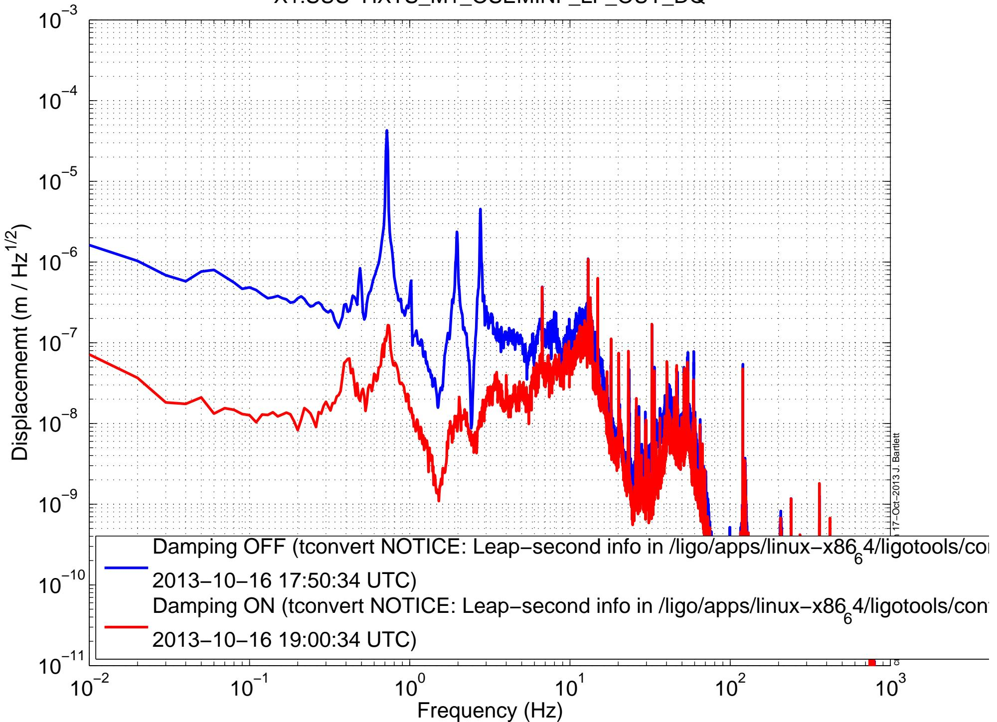
X1SUSOMC (OMCS) Amplitude Spectral Density
